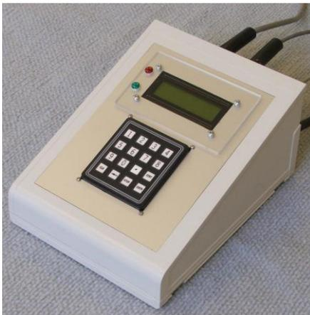
Scanning Devices' Model 755T-CS3 Repeat Length Measurement System allows you to perform this averaging with ease. It does the math for you, measuring the number of repeat lengths that you select, and then reports the average individual repeat length.
