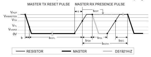
After the bus master has released the line it goes into receive mode (RX). Now, the 1-Wire bus is pulled to  $V_{PUP}$  via the pull-up resistor or, in case of a DS2480B driver, by active circuitry. When the threshold  $V_{TH}$  is crossed, the DS1921H/Z waits for  $t_{PDH}$  and then transmits a presence pulse by pulling the line low for  $t_{PDL}$ . To detect a presence pulse, the master must test the logical state of the 1-Wire line at  $t_{MSP}$ .
