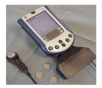
We have developed a Fleet Fueling Application for Palm Handhelds. The application allows you to read and write to DS1992L-F5 iButtons in the field.
