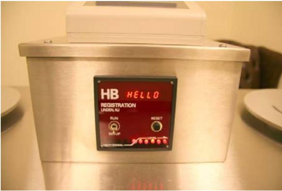
The picture on the left shows a standard Counter Display. The function of the counter is to respond to the photo-sensor at the counting station, to register counts on the light-to-dark transition (beam break) and display the current label count. The counter shows the number of times the light beam has been broken since the last counter reset. The counter also houses the Run/Setup Switch and the Counter Reset Button.
