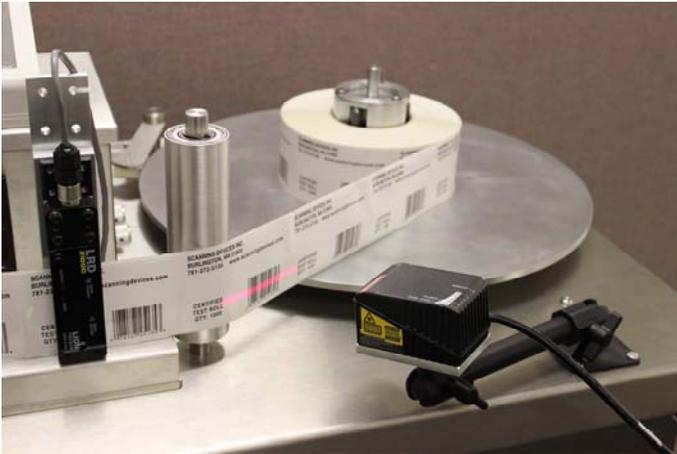
The barcode reader is a High Speed laser scanner. It uses a rotating mirror to construct a series of red scan lines. The scanner is mounted on a three-dimensional adjustable bracket, allowing the scanner to read codes with either horizontal or vertical positioning.
