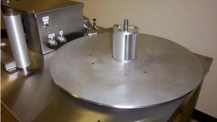
Each Scanning Devices Label Table has two 18" Lift-off label discs with 3" mechanical core chucks. It is a bi-directional machine which means it can count in both directions, or, count in one direction and then rewind the counted label roll. Both label disks are independently powered by two separate electric motors installed on the underside of the label table. When counting in the forward direction, (left-to-right as you face the front of the label table), the label disc on the right
