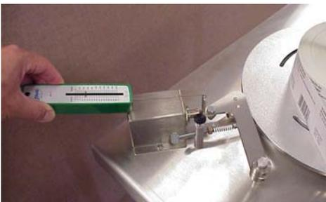
To determine the Tension setting, a “pull” tension gauge is applied to the flat riser on the Supply Reel Tension Control Arm. Tension is only adjusted on the Supply Reel, not the Take-up Reel. Once the correct tension is set, use the black locking dial to lock the adjustment screw in place.
