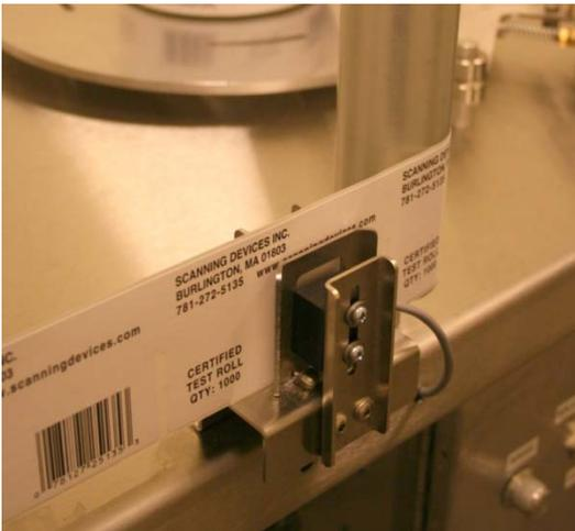
The emitted light beam is small, 1/8th inch in diameter, and the two components (emitter/detector) are mounted close together to focus on the label web. Alignment is important and is correct if the top and side surfaces of the components are in the same plane.
