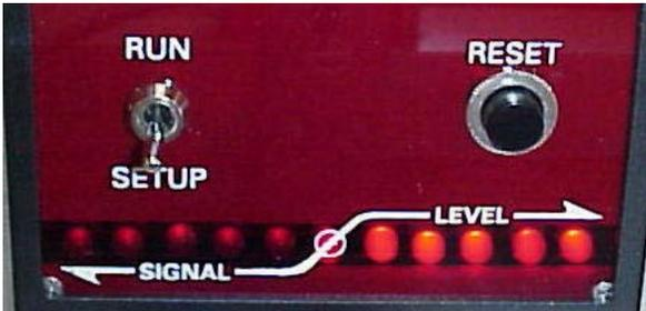
For best counting, the lights to the **right of center**, as shown in the photograph should be ON when the space between labels is positioned in the light beam (light projects through the label backing only). Adjust the sensitivity with the coarse and fine adjustment dials on the right side of the counter so that all five lights are on when the backing only is in the sensor.
