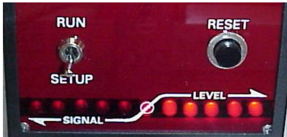
1. Setup Lights - when backing only is in the path of the sensor beam.
