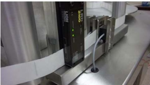
Load the clear labels on the supply reel (left side for forward direction) feed the web through the clear label sensor and the center counting station (as shown). It is important that the Clear Label Sensor switch be turned on before turning the motor speed switch on.
