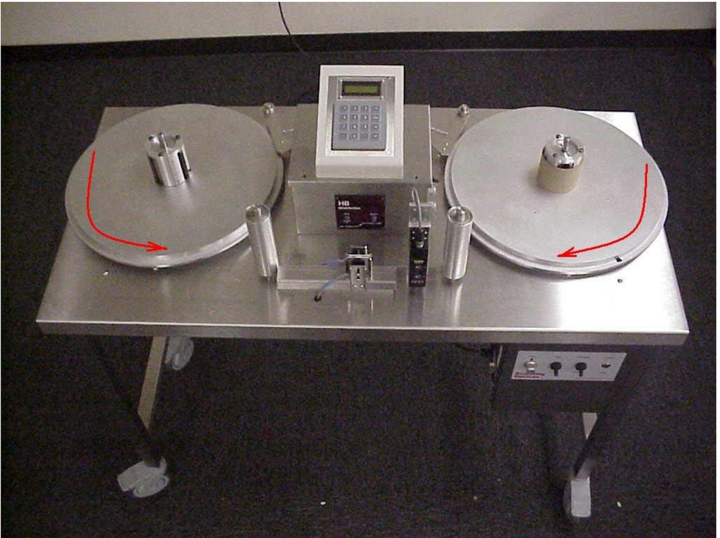
**Figure 5: Mount the label roll elevators over the core chucks and rotate until the pins reach the ends of the slots.**
