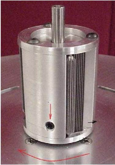
**Figure 2: Left Reel Chuck, Allen Screw Below**
