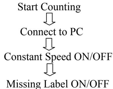
Advance through the menu features by pressing the **ENT** Key on the Label Table Keypad.
