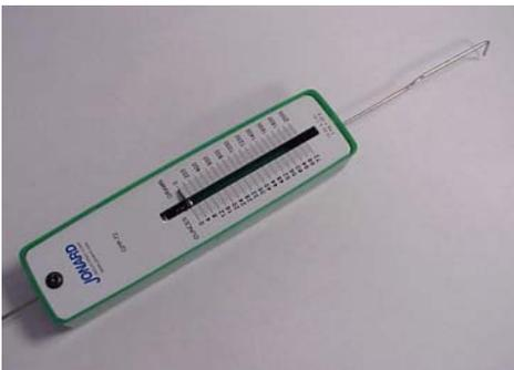
Tension Control Arms can be roughly calibrated using a push-pull tension gauge. This will assist with more consistent tension settings between rolls.
