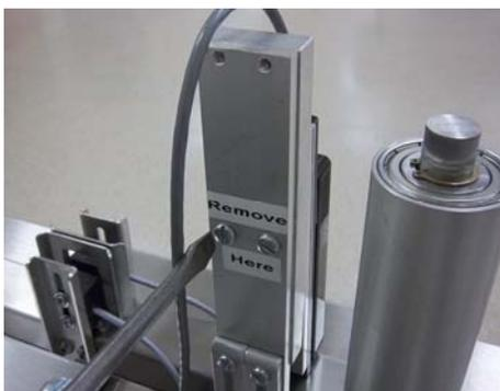
To remove the clear label sensor, simply remove the screws on the back of the Clear Label Sensor Bracket also labeled “Remove Here”. DO NOT REMOVE THE CLEAR LABEL SENSOR BRACKET CONNECTED TO THE LABEL TABLE. Once the two attachment screws are removed, the clear label sensor spacer and clear label sensor can be removed from the counting station area, and the sensor can be raised or lowered as needed.
