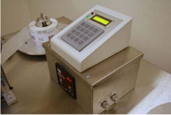
The keypad and display mounted on the center console provide an easy-to-use interface for machine start-up, operation, and other optional features. When the Label Table is first powered on it displays a menu of action options to the operator. The display consists of two lines. The keypad has sixteen keys as shown below:
