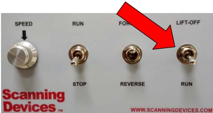
In order to remove the lift-off disks you must first release the tension control arms by lifting the switch on the front panel of the lower control box. The switch is labeled "LIFT OFF"
