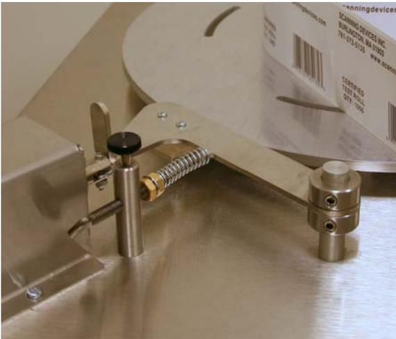
The tension control arm (two are installed on bi-directional label tables) is provided to ensure that as labels are being processed the tension of the label web remains constant. Tension is only applied to the “Supply” disk during label processing. This helps to ensure consistent label roll winding tensions and minimizes telescoping of labels as the labels are wound onto the take-up core.
