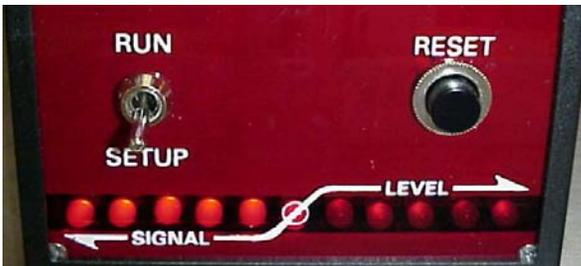
Next, move the label web so that a label is in the sensor's light beam. The lights to the **left** of center should be ON when the label is positioned in the light beam, (light beam is broken by the label material plus backing). Adjust the coarse and fine adjustment knobs to maximize the number of lights being illuminated.
