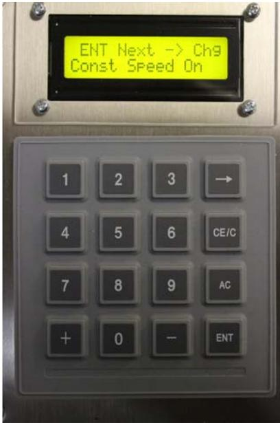
The setup menu is displayed when the Label table is first powered ON.
