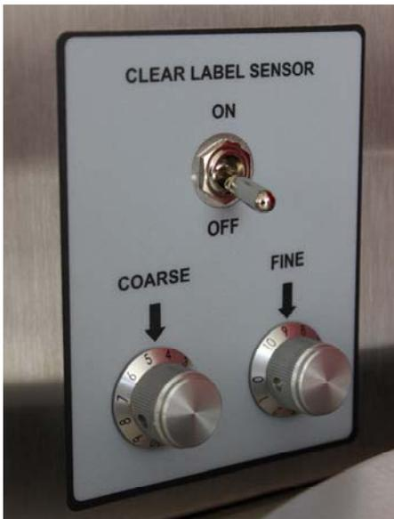
**C. Sensitivity** – changes to the sensitivity of the sensor for different types of labels and label backing materials may be necessary and is accomplished as follows:
