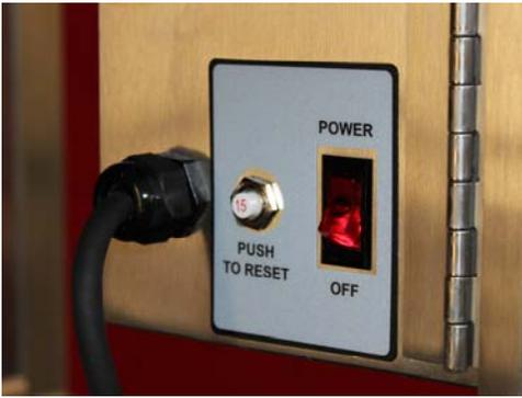
(5) **Lighted Power Switch:** controls all power to the table and is located on the left hand side of the main control box. This switch must be on to run the machine.
