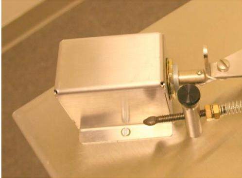
The electric brake is offered as an option on label tables with features that require fast stops of the label web for inspection of missing labels, mis-matched bar codes, or splices. The Electronic Brake will engage to stop the web when a missing label is detected. This feature will also automatically release pressure from the tension control arm and the take-up reel when counting/processing begins.
