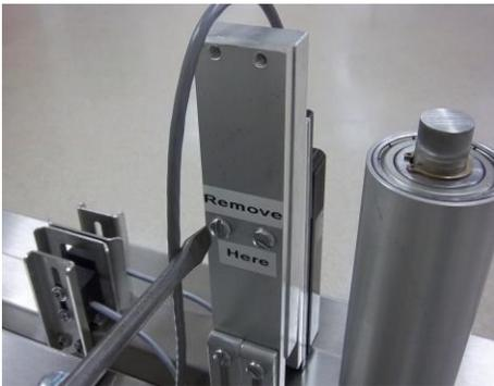
To remove the clear label sensor, simply remove the four screws on the back of the Clear Label Sensor Bracket also labeled “Remove Here”. DO NOT REMOVE THE CLEAR LABEL SENSOR BRACKET CONNECTED TO THE LABEL TABLE. Once the four attachment screws are removed, the clear label sensor spacer and clear label sensor can be removed from the counting station area, or the sensor can be raised or lowered as needed.
