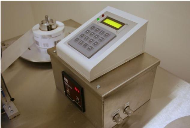
The keypad and display mounted on the center console provides an easy-to-use interface for machine start-up, operation, and other optional features. When the Label Table is first powered ON it displays a menu of action options to the operator. The display consists of two lines.
