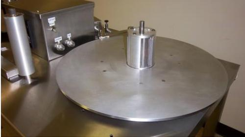
Your Scanning Devices Label Table has two 18" lift-off label discs with 3" mechanical core chucks. It is a bi-directional table which means you can count in both directions and both label disks are independently powered by two electronic motors installed on the underside of the label table. When counting in the forward direction, (left-to-right as you face the front of
