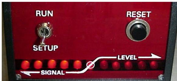
Next, move the web so that label is in the sensor's light beam. The lights to the **left of center** should be on when the label is positioned in the light beam, (light beam is broken by the label material plus backing).
