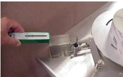
To determine the Tension setting, a “pull” tension gauge is applied to the flat riser on the Supply Reel Tension Control Arm. Tension is only adjusted on the Supply Reel, not the Take-up Reel. Once the correct tension is set, use the black locking dial to lock the adjustment screw in place.
