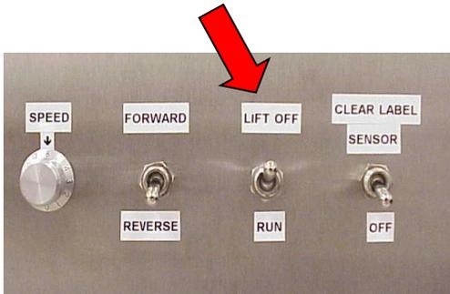
In order to remove the lift-off disks you must first release the tension control arms by lifting the switch on the front panel of the lower control box. The switch is labeled "LIFT OFF".
