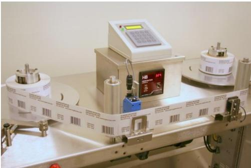
The labels to be processed are placed on the label disk on the left side of the label table (Supply Disk) with the labels unwinding from the left side, (counterclockwise rotation). The label web is fed in front of the left Label Web Guide with the backing facing the label guide. It then passes thru the counting station and across the front of the second label guide and is wrapped around a blank 3” corrugated core that is placed on the right side mechanical core
