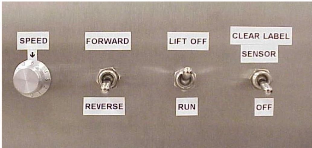
The panel hangs below the right side surface of the table and provides controls to power the table motors as well as to setting features of the table. The primary controls of a Scanning Devices Label Table are as follow from Left to Right in the picture above:
