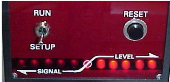
For best counting, the lights to the **right of center**, as shown in the photograph should be ON when the space between labels is positioned in the light beam (light projects through the label backing only). Adjust the sensitivity with the course and fine adjustment dials on the right side of the counter so that all five
