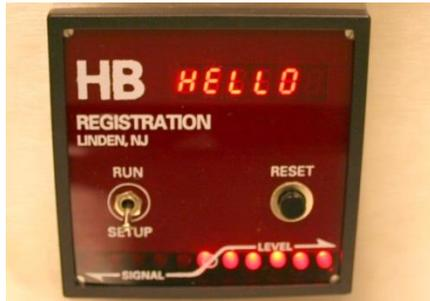
The counter's setup switch puts the counter in "Set-Up" mode allowing sensitivity adjustments for best optical contrast and sensing between label on web and spaces between labels. Adjusting the sensitivity to the specific label material being handled allows for the processing of a wide variety of label and label backing combinations.
