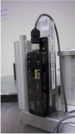
Your machine is provided with a clear label sensor shown here. This sensor is designed for counting clear labels on solid web backing or clear labels on clear web backing. The clear label sensor can be left in place when counting standard solid labels, it is recommended that the sensor is cleaned with some compressed air to remove any dust collection in the clear label sensor “sense” area.
