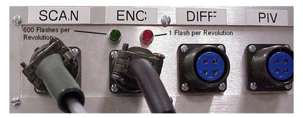
Check the scanner input (Yellow light on the Quarter-trol Panel). It should flash once per machine revolution.
